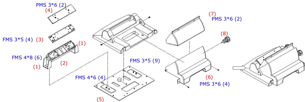
To assemble the pedestal set to the panel PC, simply retain them together with four PMS M4\*18 screws from the base. Then, fix the stand upper cover (7) to the panel PC with two PMS M3\*6 screws. The stand can be tilted from 45 to 90° by swiveling the base knob (8) and pulling the base up and down.
